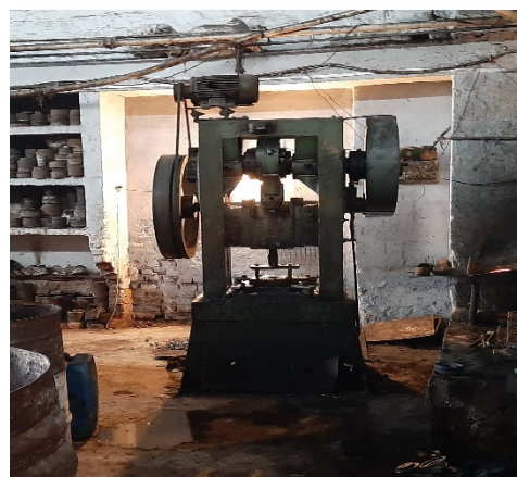
Figure 3: Working power press at forging unit
